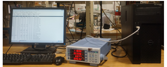
Fig. 5: Tapping an AC electrical outlet.
