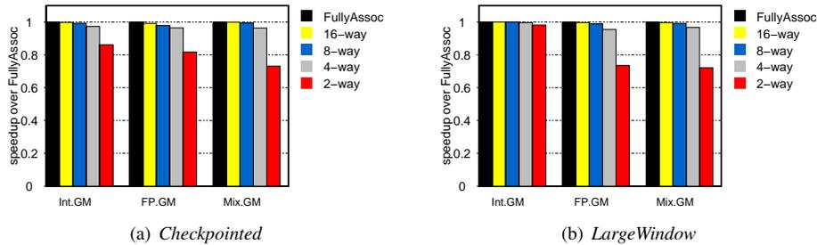
Fig. 7. Effect of varying the associativity of a 32-entry MHA.
