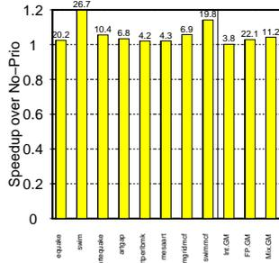
Fig. 10. Performance impact of memory request prioritization in the *Checkpointed* processor. The numbers on top of the bars refer to the percentage of bus requests that were assigned high priority.
