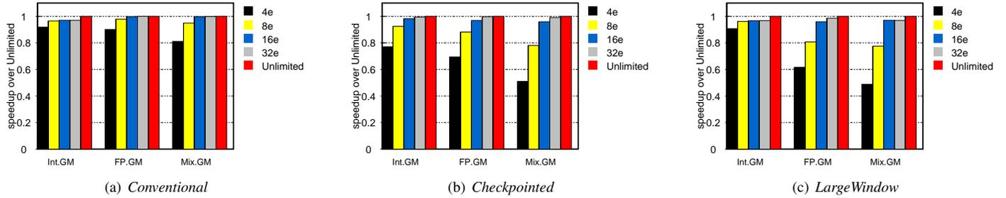
Fig. 5. Effect of varying the number of MHA entries.
