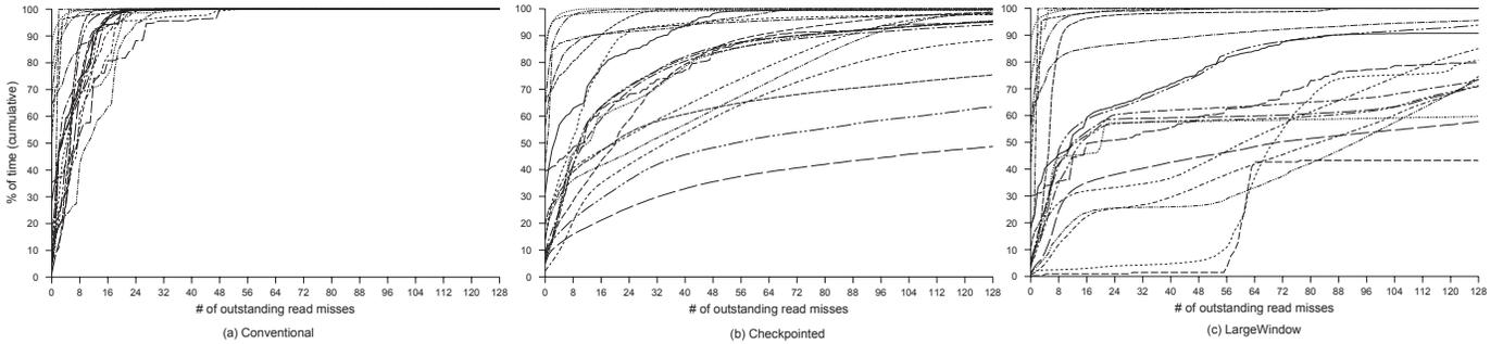
Fig. 2. Number of outstanding L1 read misses at a time in *Conventional* (a), *Checkpointed* (b) and *LargeWindow* (c).
