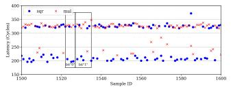
Fig. 16. Access latencies measured in the reload operation in Evict+Reload. A sequence of "0101011110110101" can be deduced as part of the exponent.
