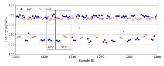
Fig. 14. Access latencies measured in the reload operation in Flush+Reload. A sequence of "1001110101" can be deduced as part of the exponent.
