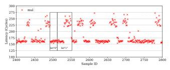
Fig. 15. Access latencies measured in the probe operation in Prime+Probe. A sequence of "01010111011001" can be deduced as part of the exponent.
