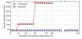
Fig. 7. Target line access latency as a function of the number of eviction addresses in experiments to analyze the inclusive property for private lines.
