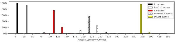
Fig. 5. Latency of a cache line access when the line is in different locations in the Intel Skylake-X cache hierarchy.
