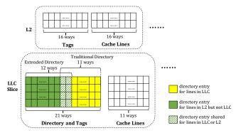
Fig. 9. Reverse engineered directory structure.
