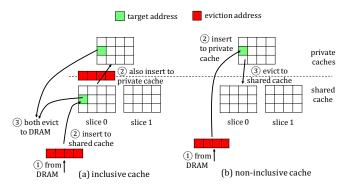
Fig. 4. Attempting to evict a target line in inclusive (a) and non-inclusive (b) cache hierarchies. Victim and attacker run on the same core.
