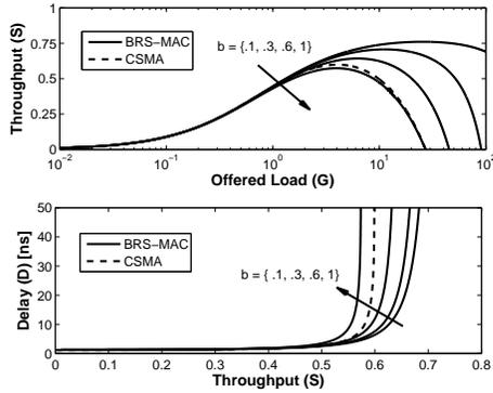
**Figure 5: Throughput and delay as functions of the position of the preamble.**
