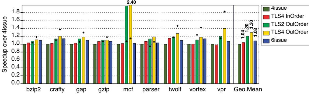
Figure 6: Speedups of different binary-architecture combinations relative to *BaseApp* running on *4issue*. The figure also shows the geometric mean. The TLS results are obtained with a fully-automated TLS compiler on full SPECint applications.
