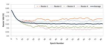
**Figure 7:**  $V_{dd}$  of different routers stabilizing over time. There is wide variation in the final  $V_{dd}$  of different routers across the system.
