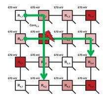
Figure 3: Slow routers are at the intersection of many faulty paths.
