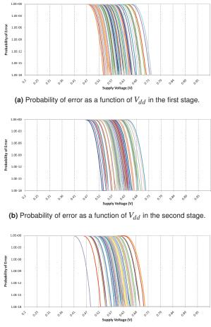
(c) Probability of error as a function of  $V_{dd}$  in the third stage.
