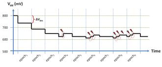
Figure 1: Changes to the  $V_{dd}$  of a router over time in Tangle.
