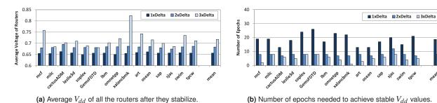
Figure 12: Effect of varying  $\Delta V_{inc}$  on the average  $V_{dd}$  obtained, and the number of epochs needed to obtain stable  $V_{dd}$  for the routers in an 8x8 Tangle NoC.
